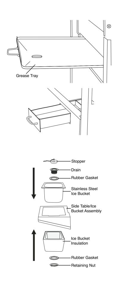
Insert grease tray into opening on backside of grill. Make sure to slide tray onto tracks as illustrated.
